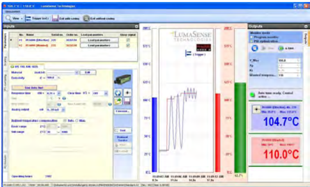
Measurement with Internal Temperature of radiation temperature and internal instrument temperature. Parameters can be changed during the measurement.
