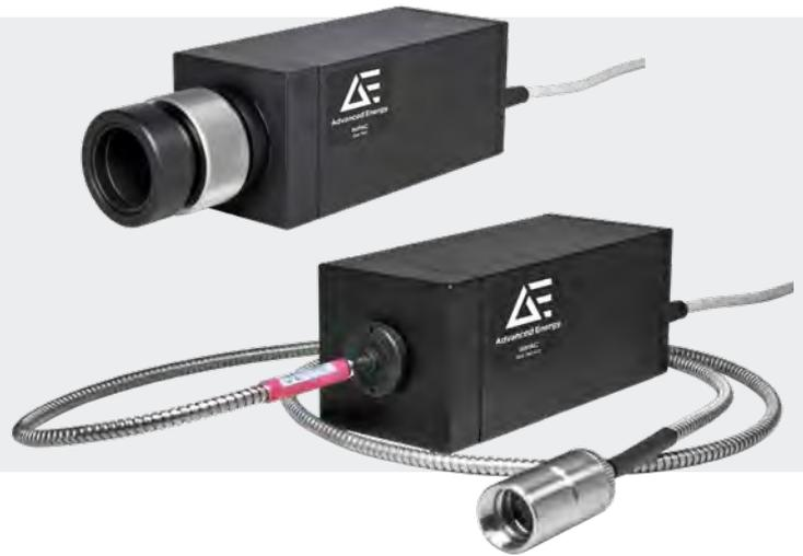
The Impac® IGA 740 and IGA 740-LO pyrometers are stationary instruments specifically designed with an extremely fast response time of only 6  $\mu$ s, making them suitable for monitoring fast moving objects or fast temperature changes. The pyrometers are also available as temperature measuring stations IMGA 740 and IMGA 740-LO.
